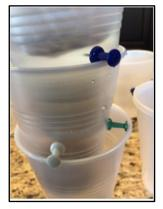
To build the stackable water filter, students will take 5 cups and use the push pin to punch holes in the bottom of each cup so the water can pass through. The sixth cup will be used to collect the water, and it represents the bedrock. Have students use push pins on the side of each cup to create the stackable filter.
